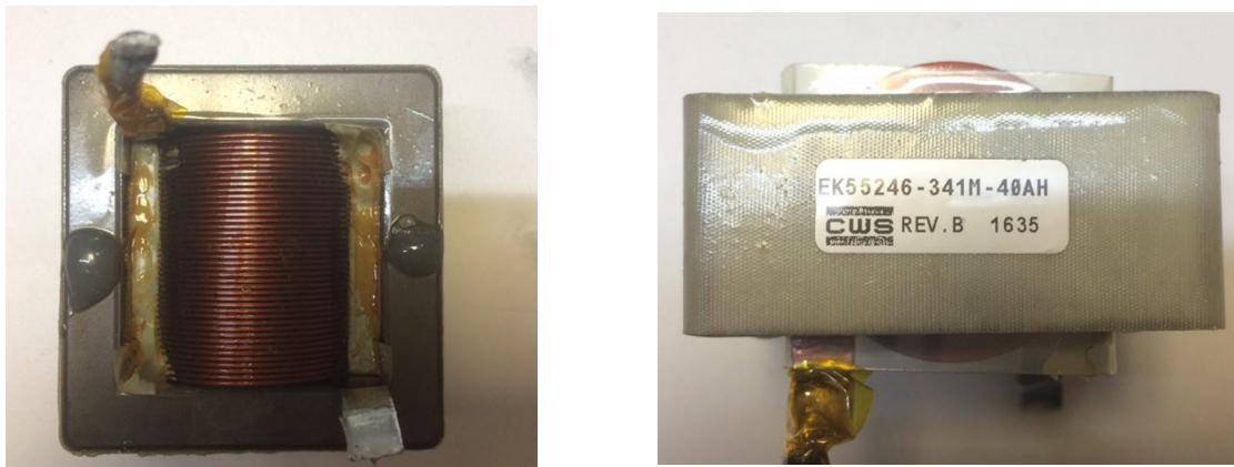
Figure 8. Load Inductor Example
