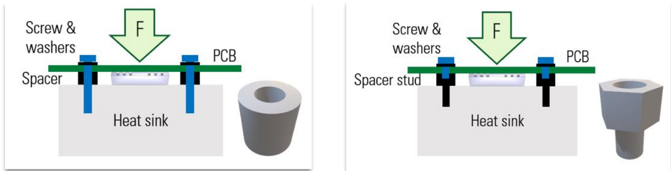
Figure 10. Mounting the SMPD using Cylindrical Spacers or Screw-type Spacer Studs
